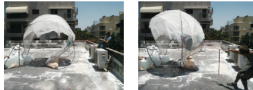
Structural test of horizontal and twisting loads. The tester holds a digital spring scale which provides an accurate reading of loads. Each test lasted about an hour, using both manual and tester tools only exposure.
